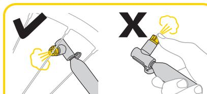
After each inflation, make sure all CO<sub>2</sub> gas has been discharged by pushing the AirBooster inflating head several times.
