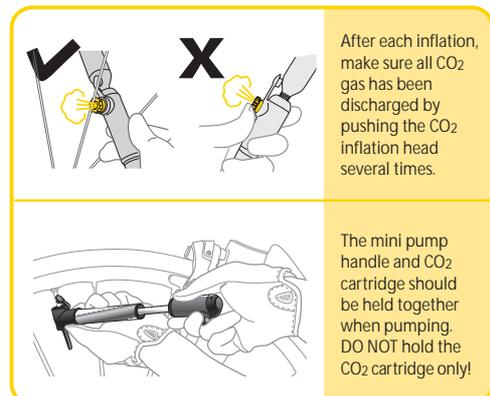
After each inflation, make sure all CO<sub>2</sub> gas has been discharged by pushing the CO<sub>2</sub> inflation head several times.
