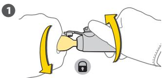
Thread CO<sub>2</sub> cartridge clockwise until full engagement is achieved. Be careful not to cross thread the CO<sub>2</sub> cartridge.
