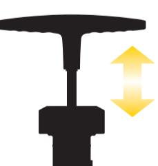
Pump to desired pressure. Press the Air Release Button to adjust the pressure as necessary.
