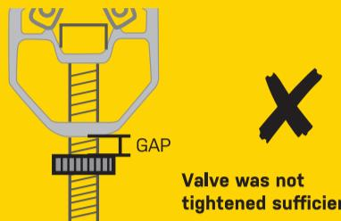
Valve was not tightened sufficiently.
