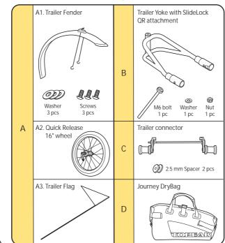
\* Tools Required: 4mm Allen key, 5mm Allen key, 10mm open end wrench
