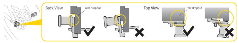
2 Make sure the hook of Trailer connector is installed in proper position on both sides.
