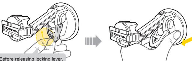
Before releasing locking lever, please check the space is enough to release CarMount from surface as shown.
