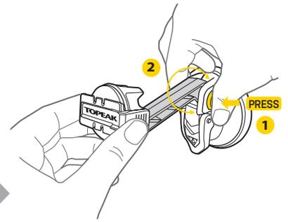
4. Press the angle adjusting knob to adjust the car mount vertical angle.
